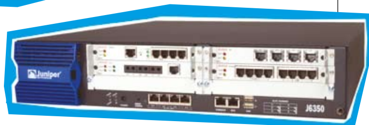
Avaya IG 550 Gateway in Juniper J6350 Router
